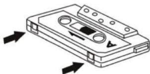
**Note:** Make sure that the erase prevention tab on top of the tape has not been cut off. If these tabs have been removed, the tape cannot be used for recording.
